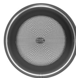
CircLED 2BE 016 540-011 Direction Indicator, DRL and position lamp (10-32V) DT Connector
