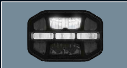
Low beam and position light
