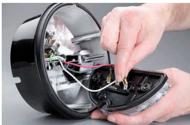
Step 4: Connect the LED module and flat receptacles. Please observe the correct pin assignment and sequence: Black = taillight Red = stop lamp White = ground
