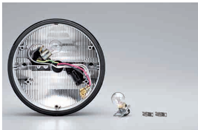
Step 3: Loosen the flat receptacles from the contacts and remove the bulb together with the bulb holder
