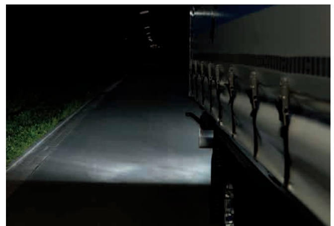
Illumination with additional reversing spotlights
