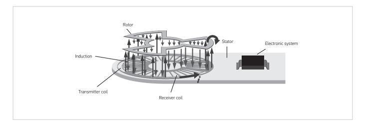
Inside the laser-welded polyamide housing (PA66), the rotation of the lever arm is transferred to the rotor and measured by induction. An ASIC (Application Specific Integrated Circuit) accurately computes the rotor position. Various mounting positions are possible thanks to the repeating characteristic curve of the output signal (which depends on the structure of the sensor that is used), which increases the flexibility of the sensor.
