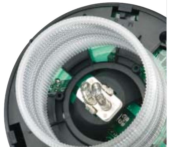
Simple interior lens; low EMC protection measures
