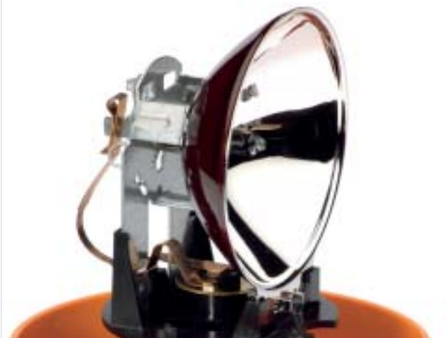
Bulb and reflector form a rotating unit
