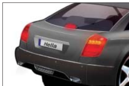
ECE 2-stage brake light: daytime level
