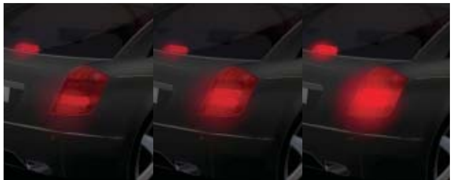
Demonstration of the different levels for the dynamic braking signal (DBS)
