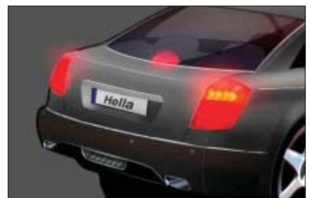
ECE 2-stage brake light: night-time level
