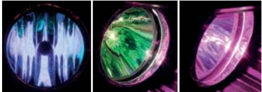
Figure 3: Initial samples of an infrared headlamp using a halogen bulb and interference filter. The typical angle-dependent color play of such filters can be seen.
