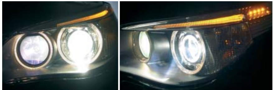
Figure 4: Current status of infrared modules (on the left each time) integrated in a prototype on the basis of a Bi-Xenon series device.
