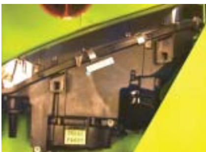
Fig. 4: Headlamp during impact, taken from a high-speed video
