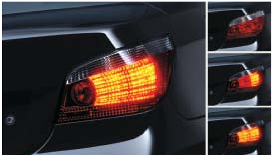
Fig. 2: Hazard stop signal by increasing the signal area (BMW)
