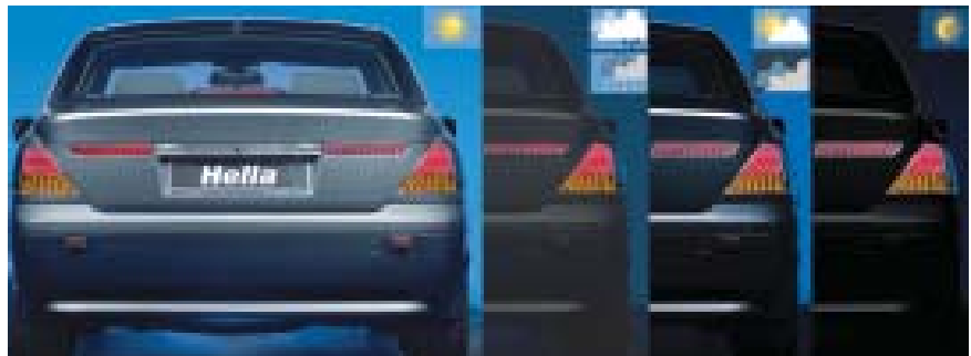
Fig. 3: Adaptation of the signal image to different ambient brightness
