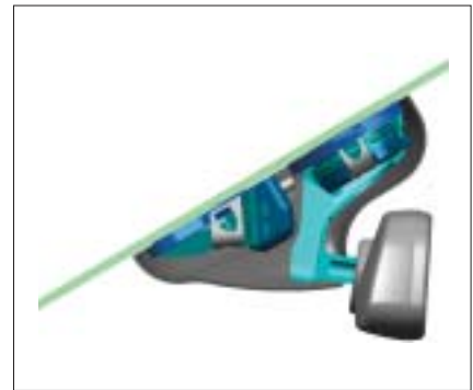
Integration of camera + rain/light/solar sensor in the mirror base
