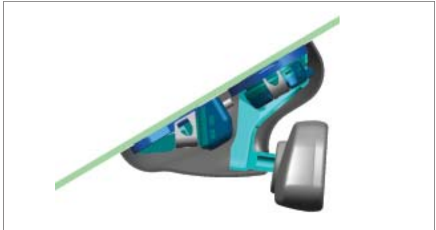
Lane departure warning camera and rain/light sensor integrated into the mirror base
