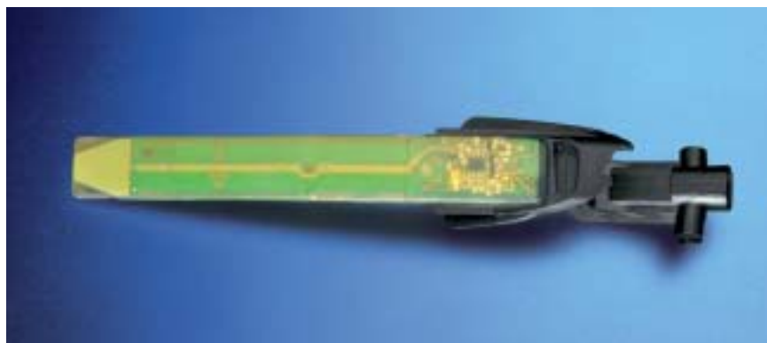
Rear door handle sensor technology
