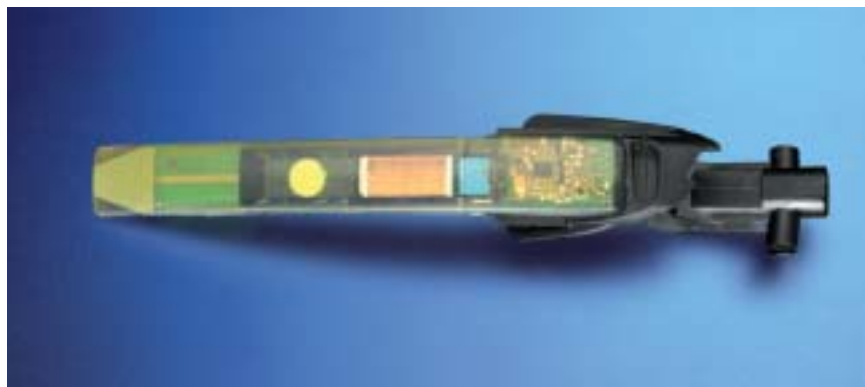
Front door handle aerial/sensor technology
