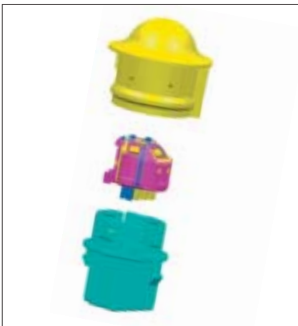
Structure of the sun sensor with standardized component part carrier using MID technology
