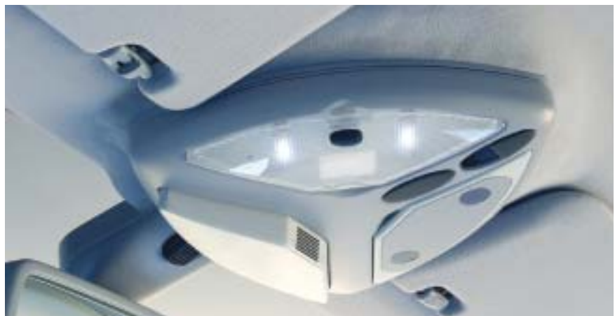
Three differently interchangeable modules in the overhead electronics
