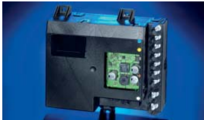
Charge converters from Hella integrated into a vehicle electric system control unit
