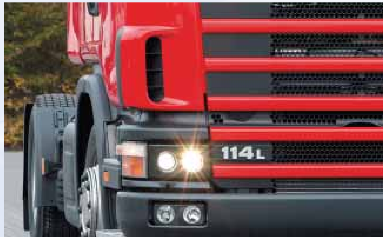
Road illumination with halogen low beam light
