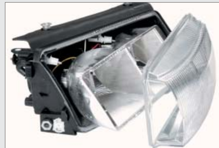
The broken reflector brackets of the test subject can be clearly recognised.
