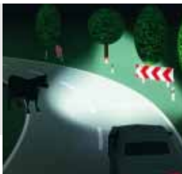
When driving around bends, obstacles on the inner radius of the bend are always difficult to see.
