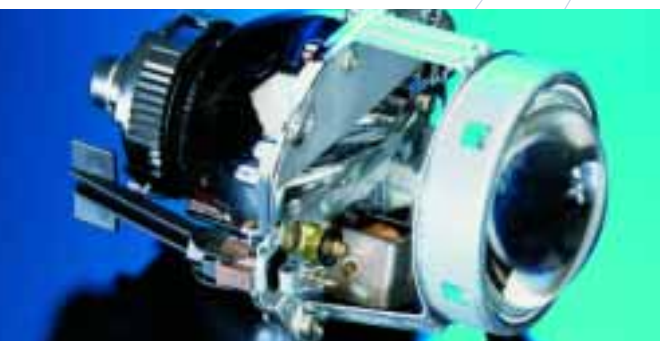
Headlamps with bi-xenon module. Dipped beam light and main beam light from only one xenon bulb.
