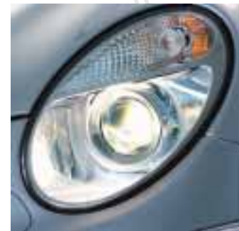
All xenon and bi-xenon systems have an integrated dynamic headlamp leveling device and headlamp cleaning system.
