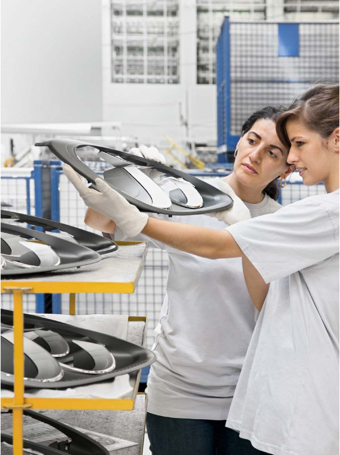
Headlamp cover frames are inspected before being allowed to continue to the next processing stage.
