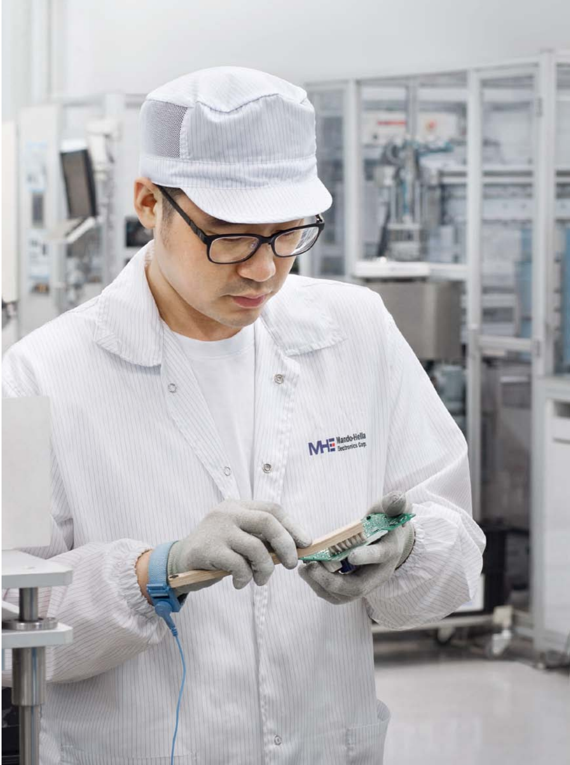
Excess material is brushed from the PCB for an electric servo-assisted steering system after soldering.
